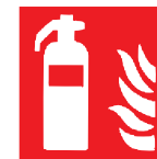
F001 Fire extinguisher
