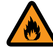
W012 Warning: Flammable material
