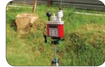
Figure 10.2: WBGT monitor (including Globe thermometer).
